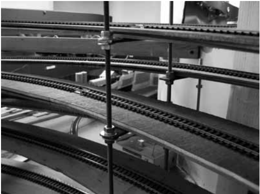
Bruce uses threaded rods and metal crosspieces to support the helix sub-roadbed. Because the helixes climb in opposite directions, a series of "windows" is created for access from within at points around the helixes.
